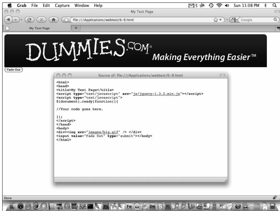
Figure 6-9: Web page with a button and a <div> element containing an image.
